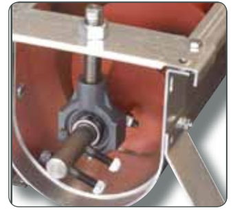
Auger suspended in adjustable ball bearings
