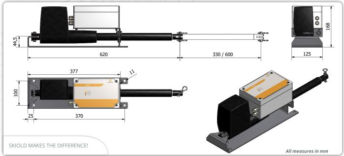
Used to open/close wall- and ceiling air inlet valves. Also used for emergency opening. Suitable for up to 70 wall-/ceiling air inlet valves per servo motor.
